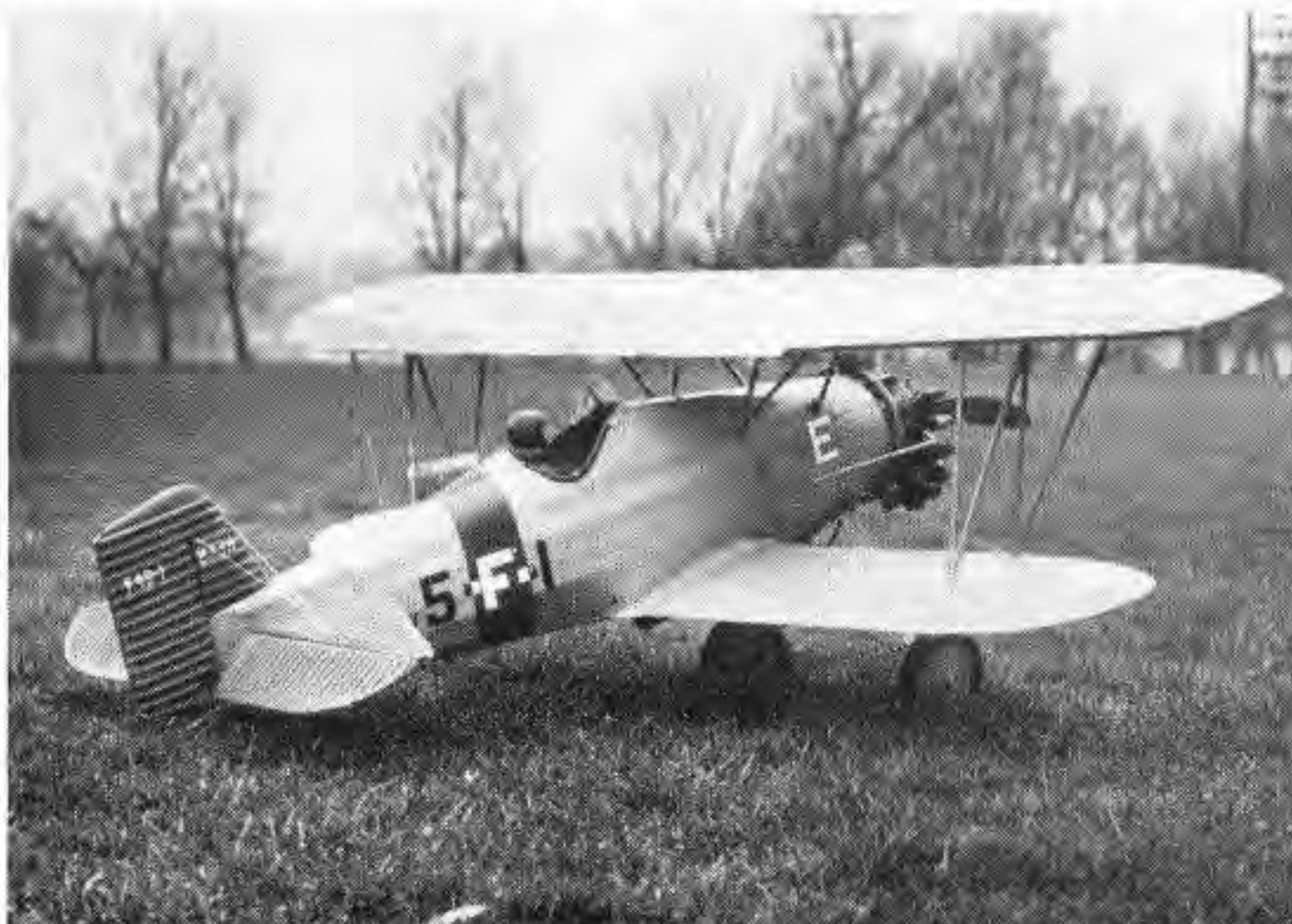
A 45in. span Boeing Model 100 built by the author for a Fox 40S R/C. Apart from the corrugated control surfaces, this model is very simple to build. Capable of loops, it also handles well on the ground – even on grass.
